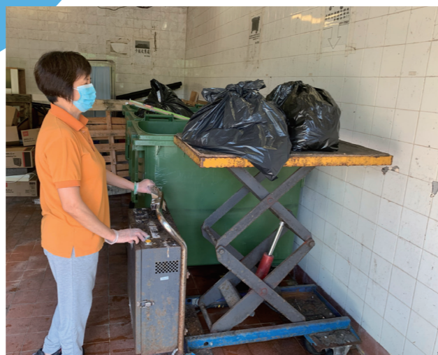
只要按下按鈕，整個升降台便會升至與高身垃圾桶高度一樣。 Press the button and the entire lifting platform can rise to the height of a tall rubbish bin.
