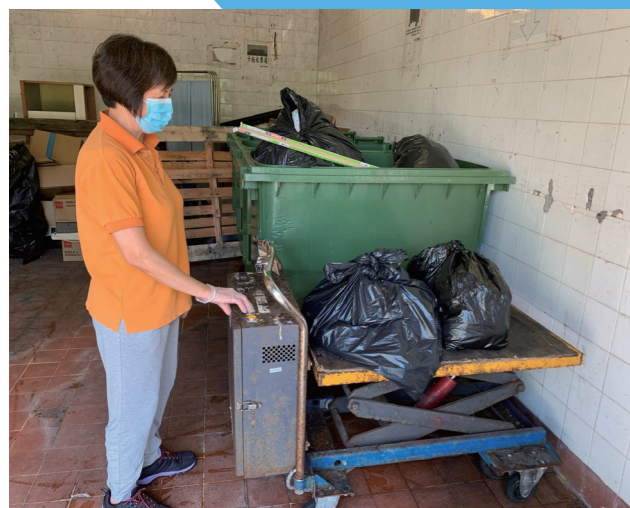
不鏽鋼面板，垃圾更容易推入高身垃圾桶內。 Using stainless steel panel, rubbish can be easily pushed into tall rubbish bins.
